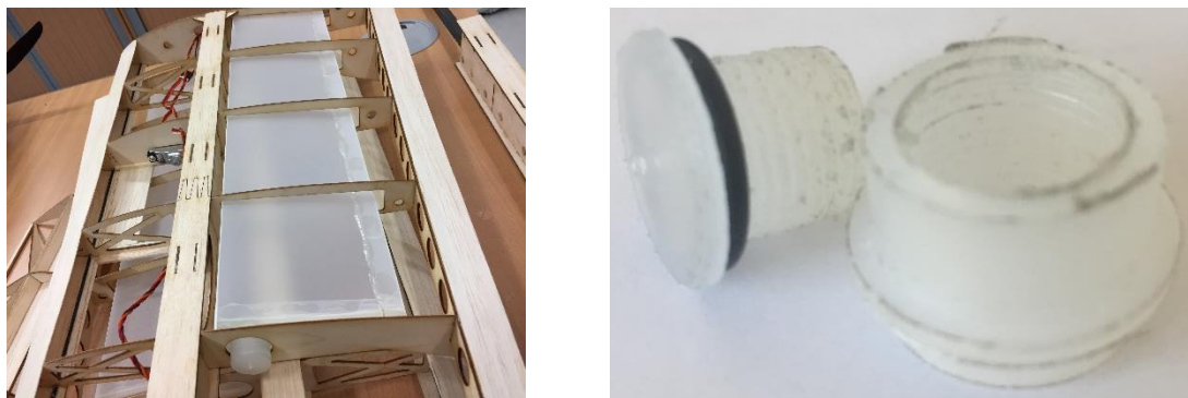
Figure 5.11 Manufactured wing tank (left) and lid (right).
