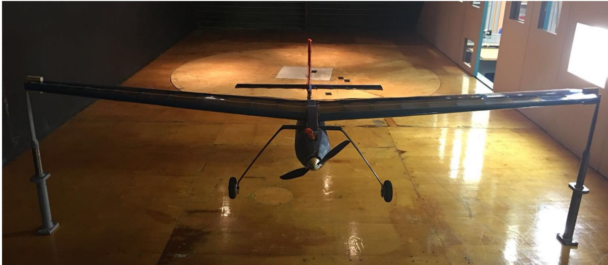
Figure 6.3 Wind tunnel test set up.
