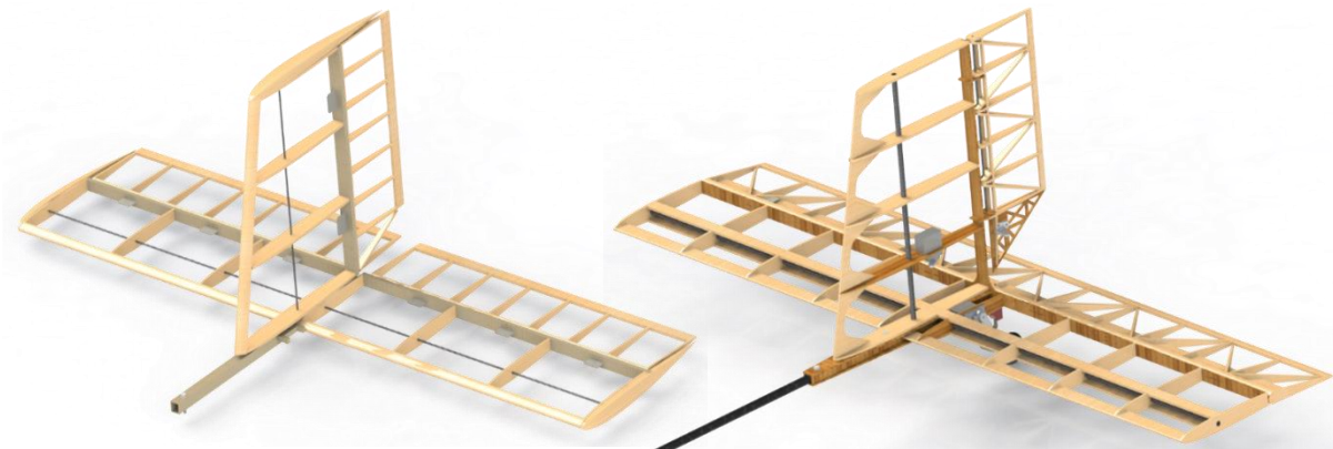
Figure 5.9: V1 (left) and V2 (right) Tail plane Assembly's.
